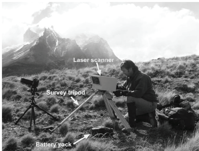
Fig. 12. A typical field setup in Patagonia in early 2002. All equipment was transported in a backpack by a single person (picture courtesy of Jeremy Willson, Shell Oil). Lithium Ion batteries have helped reduce battery weight to 1,540 grams (3.4 pounds) per approximately 2 hours of continuous scan time (Bellian et al., 2005)
