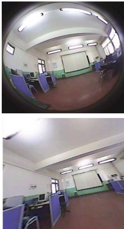
Fig. 4. A fisheye image (above) and the corrected result of a fisheye image (below)
