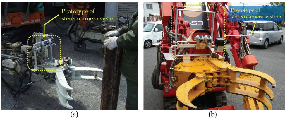
Fig. 4. Installation of the system: (a) the system mounted on the right gripper of T-52; (b) the system mounted on the right gripper of T-53.
