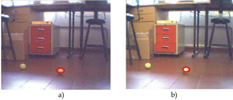
Fig. 10. Application of the CAMSHIFT algorithm to real, clutter environment. a) Presence of a distractor element. b) variations in lighting conditions.
