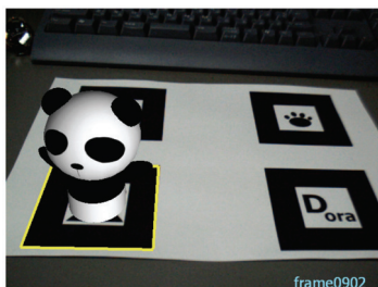
Fig. 1. Multiple markers aligned with ordered arrangement
