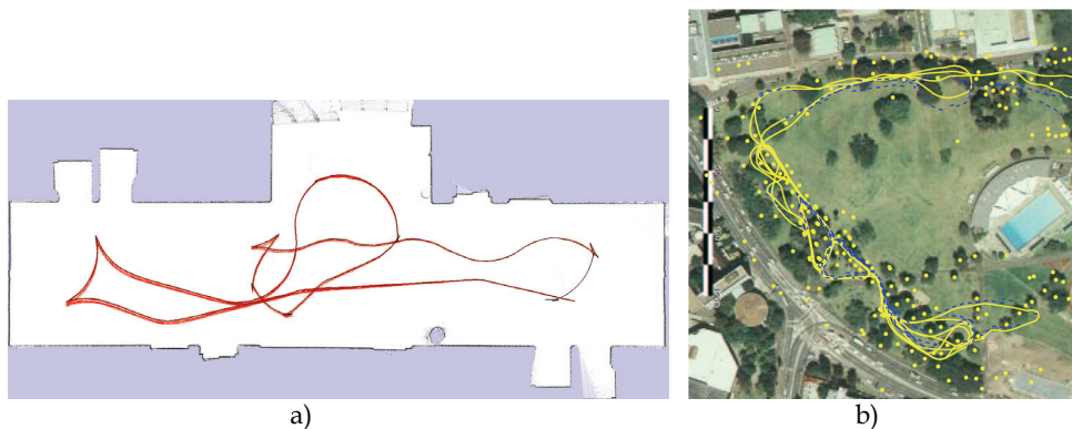
Fig. 1. Two typical maps. Fig. 1(a) occupancy-grid map. Fig. 1(b) landmark-based map: landmarks are indicated with (grey/yellow dots).
