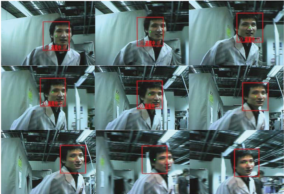
Fig. 9. Running sequence tracked with panning camera control.
