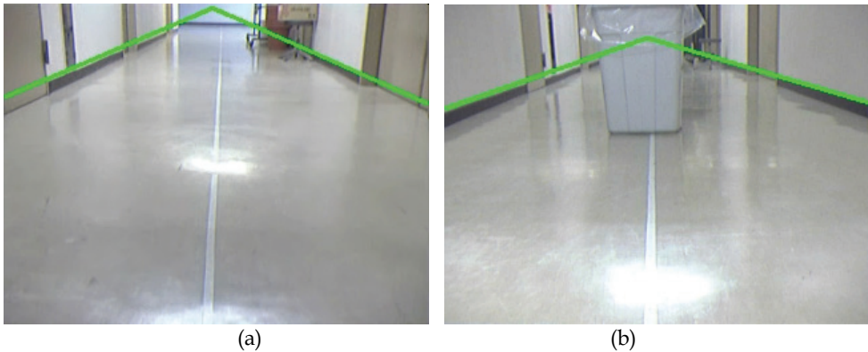
Fig. 6. Detected boundary lines of Fig. 2.
