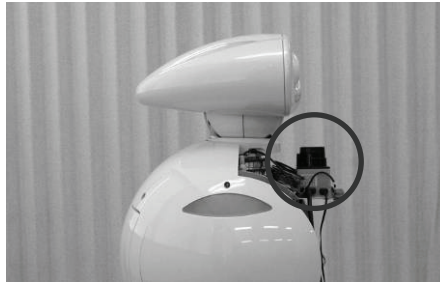
Fig. 11. LRF on ApriAttenda™ (side view)
