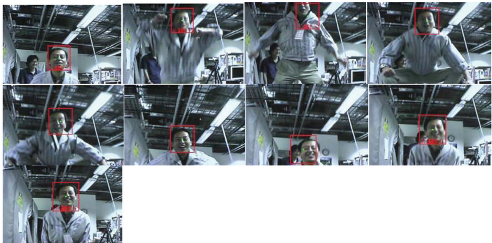
Fig. 10. Jumping sequence with motion blur, tracked with tilting camera control
