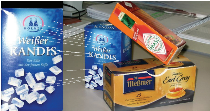
Fig. 1. SIFT feature matches applied to a self recorded scene. The blue sugar box on the left side of the image was found in the right complex scene. The SIFT matching software yielded 16 matches (shown as white lines). Note that only 3 matches would have sufficed to correctly identify an object. Also note the partial occlusion and difficult lighting conditions under which the images were taken. The digital camera used to record both images was a Canon Powershot A75 with 3.2 megapixels. The camera was set to automatic mode. The images also underwent a lossy JPEG compression.
